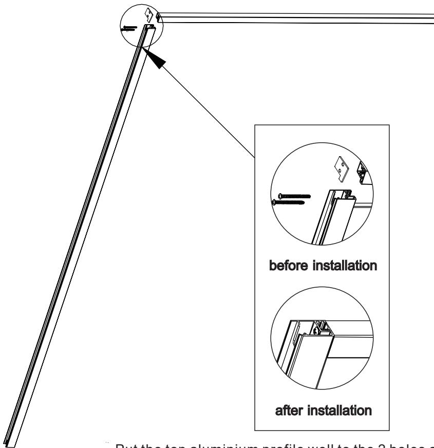
Put the top aluminium profile well to the 2 holes of front hinge profile
